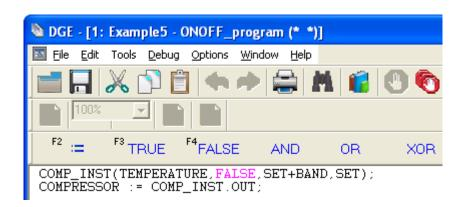
It is very important to understand that the list of the inputs is not random; the sequence of the inputs must be like the sequence of the instance.
