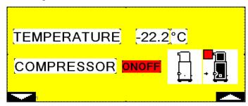
For these two images the flag "ScrollLock" have to be checked; in this way the images will be replicate automatically in all the pages of the stage (also the buttons control will be the same in all the pages).
