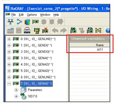
To link the variable with the board, select the "ID point" in the board:
