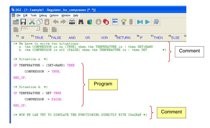
In the example here above, the variables are not linked with the physical output; these variables are only logical. To link these variables with the physical output we have to write another program.
