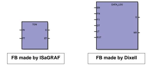
The FB is composed by some Inputs (on the left side) and some Outputs (on the right side). When you use the FB in your program is enough to send them only the value of the variables to get the result; it is not necessary to know what happen inside the blocks.
