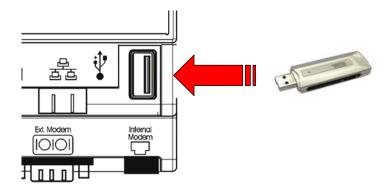
When the yellow led will blink, the file has been downloaded or uploaded; now you can remove the USB key.
