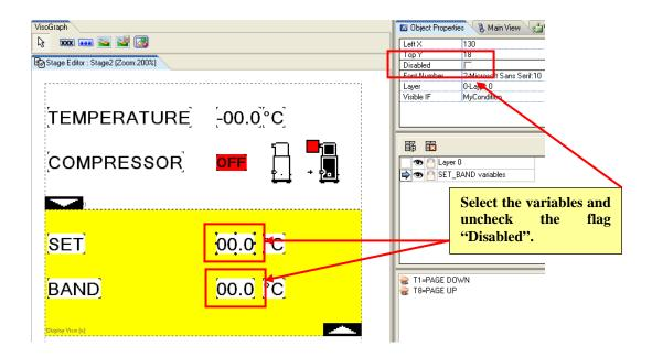
It is also possible to define the range limits; practically you can decide the range min and max of your variables. Then in the VISOGRAPH you can choose the value between min and max range. Select the variable in the page and, in the Variables properties, write the limits:
