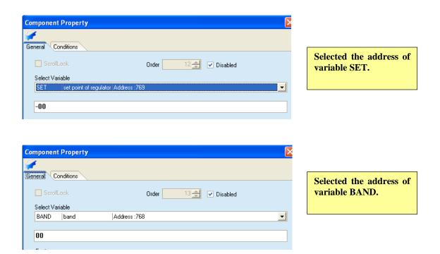
It is very important to pay attention to the flag "Disabled"; if the flag is checked the value is non modifiable with the VISOGRAPH. If the flag is unchecked the value will be modifiable through the VISOPROG buttons.
