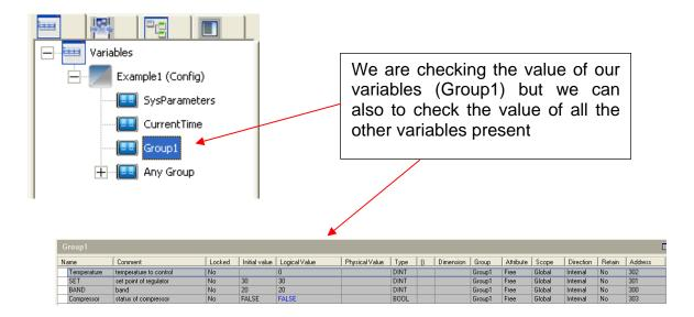
We can force the value of the input; for example we want to switch on the compressor. Double click in the box of Logical Value of the temperature: try to insert the value "60" and then confirm with "Write":
