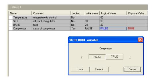
Here above the information are very clear; in our application the compressor should be on (TRUE) but, due the variable lock as FALSE, the compressor is off. Now you can change all the other variables and in any case the compressor will be off.
