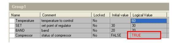
It is also possible to lock and unlock the variable; for example we can lock the variable of compressor. During the test, to avoid to damage the compressor, we can lock the compressor in off (variable must be FALSE) and then change all the other variables to understand what happen in all the other resource of our application (fan, pump, valve,...).
