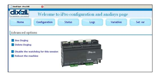
If necessary is possible to change the IP address; click the Configuration button and in the IP box write the new address (for example if your IP address is: 192.168.0.233).
