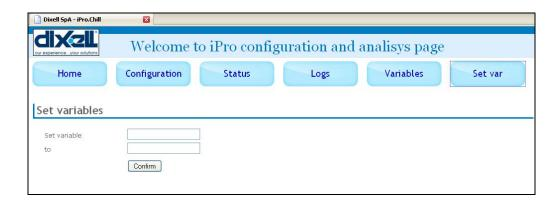
If you want to change the value of the variable "SET" from 100 to 150, write the name of the variable, the new value and then confirm.
