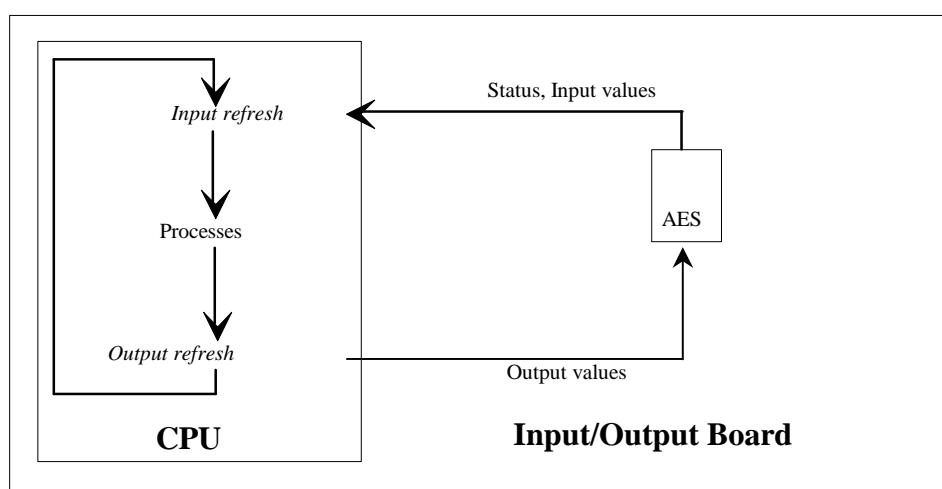
**Figure 2: Alto ISaGRAF Processing Cycle**
