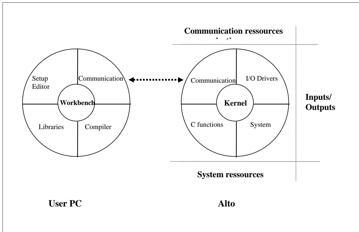
**Figure 1: ISaGRAF Architecture on Alto**
