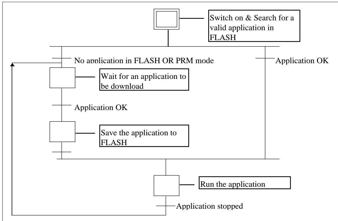
**Figure 4: Alto ISaGRAF: Theory of Operation**
