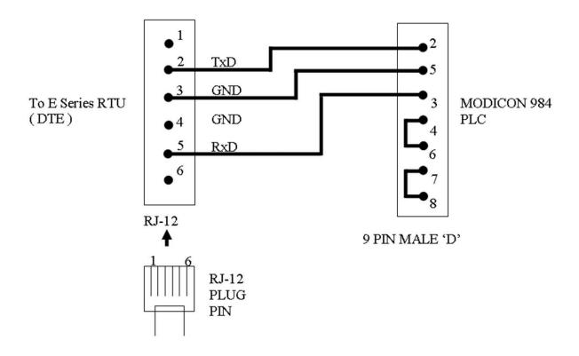
Figure 9.1: SCADAPack ES RTU to PLC Cable
