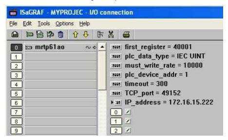
Figure 6.3: ISaGRAF Modbus RTU in TCP output board
