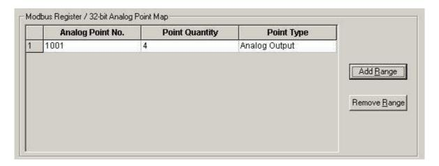
This configuration would result in the consistent register / point mapping as shown in the following diagram, irrespective of the protocol reference number (register address) and the word count specified in a Modbus request.
