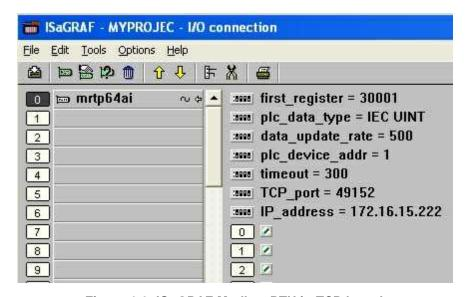
Figure 6.2: ISaGRAF Modbus RTU in TCP board
