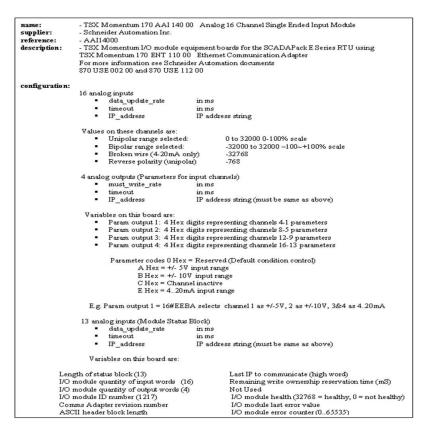
Figure 8.6: ISaGRAF "aai14000" Complex Equipment Technical Note
