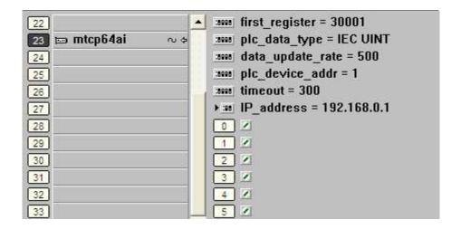
Figure 6.1: ISaGRAF Modbus/TCP board
