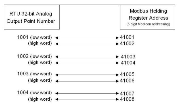
Example: a Modbus request to write to the holding register pair 41005/41006 would result in controlling RTU analog point 1003. Without the additional mapping configuration shown above, this control would have otherwise mapped to analog point 1005.
