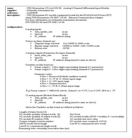
Figure 8.5: ISaGRAF "aai03000" Complex Equipment Technical Note
