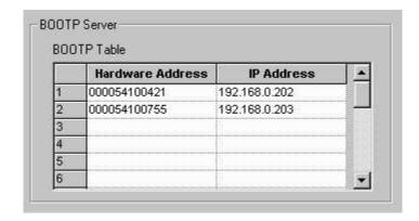
Figure 9.2: SCADAPack E Configuration of the BootP Table
