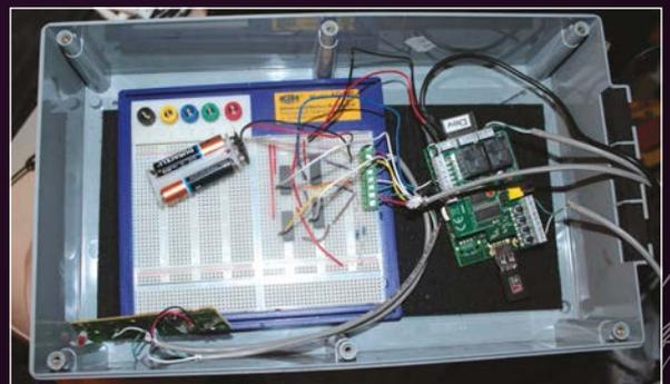
**Below** A simple box contains the Pi and all the electronics so that it's kept waterproof
