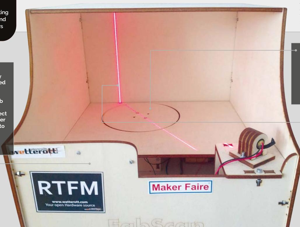
The wooden case contains a motorized turntable that rotates the object being scanned. It is currently controlled by an Arduino, although a custom Pi HAT is being developed
