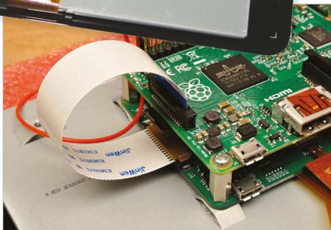
you need to safely secure it to your Pi, a DSI ribbon cable, and four jumper wires for both power and communications. Pimoroni has also produced an excellent Pibow-esque bezel with integrated stand in different colours. For a small premium, you can add your chosen colour to the shopping basket so you don't have to worry about propping the screen up or 3D-printing your own solution.
