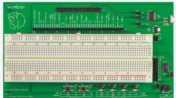
Provides **easy access** to all GPIO pins
