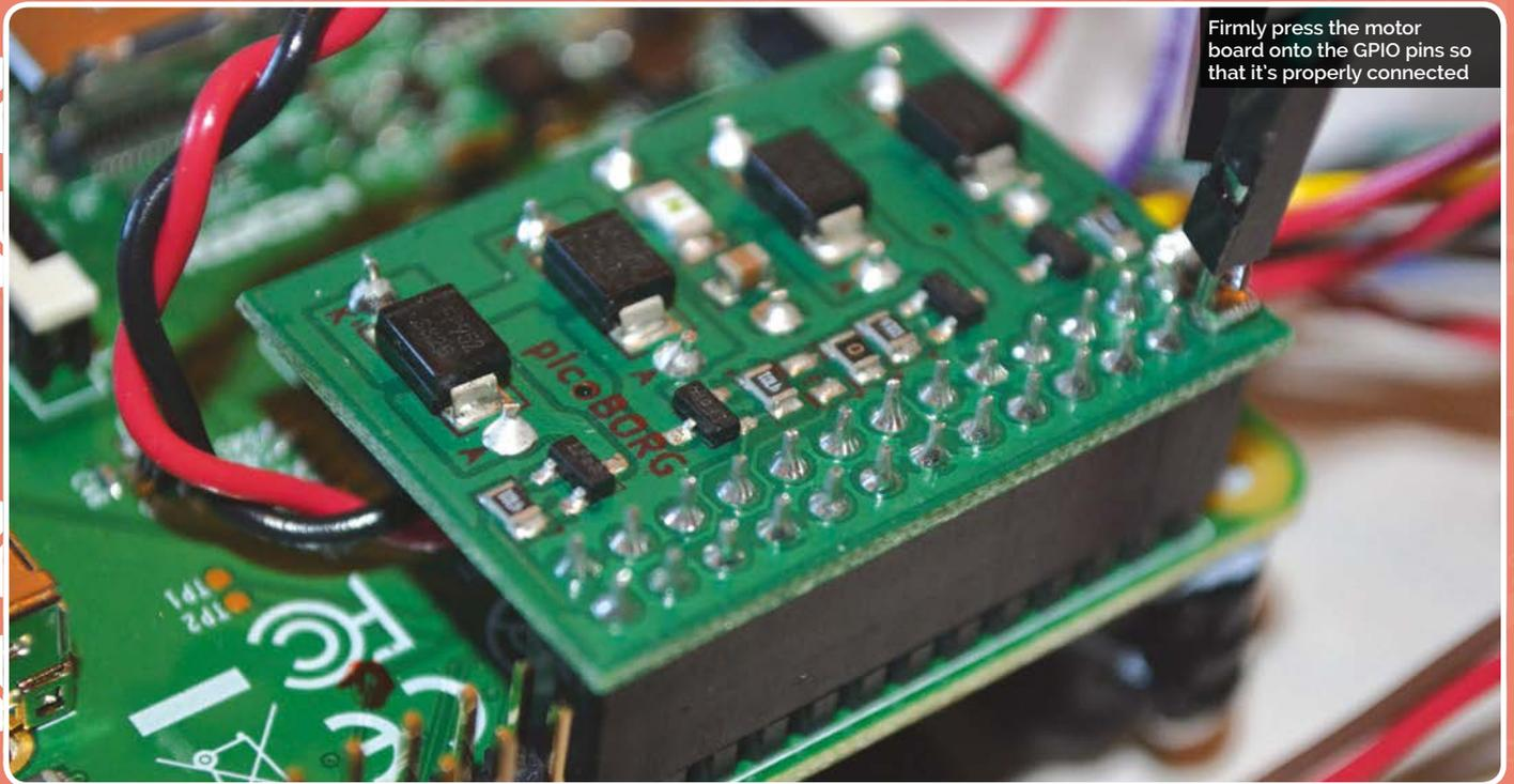
Firmly press the motor board onto the GPIO pins so that it's properly connected
