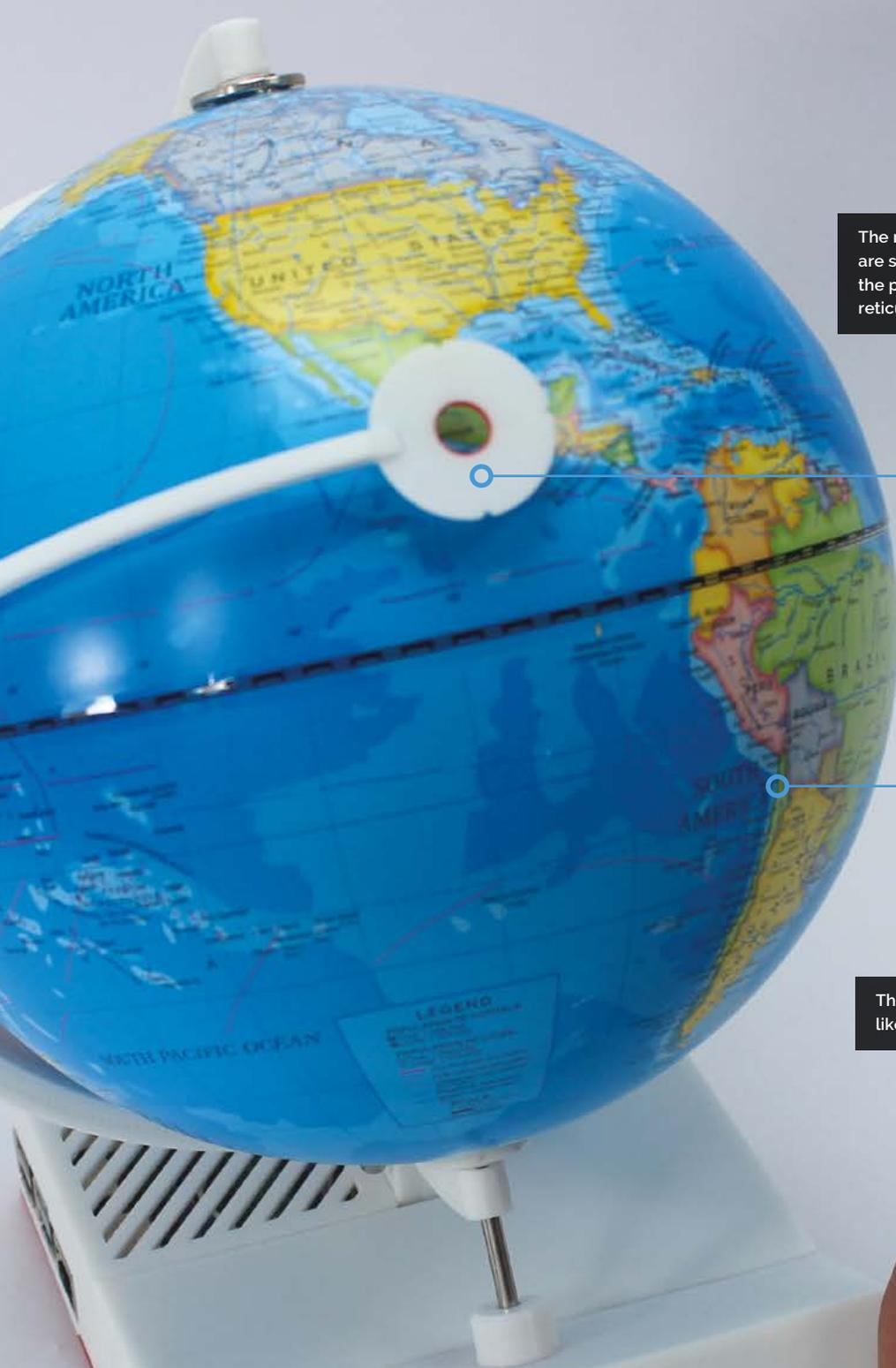
The rotary encoders are set so they know the position of the reticule over the globe
