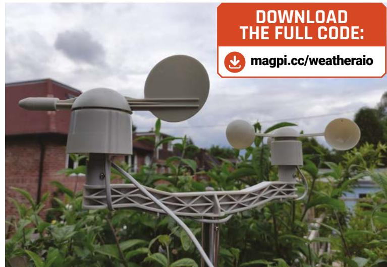
the vane is pointing toward the protrusion nearest where the main cable (going to the HAT) comes out, it's pointing north. You can double-check this by running the **weather.py** demo code and rotating the vane so it reads north.
