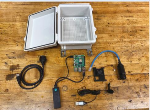
**01** A waterproof housing, Raspberry Pi, microphone, fan, and cables make up the basics of an in-the-field BirdNET-Pi station. Photos from Bill Powers' setup ([magpi.cc/birdnetbuild](http://magpi.cc/birdnetbuild)).
