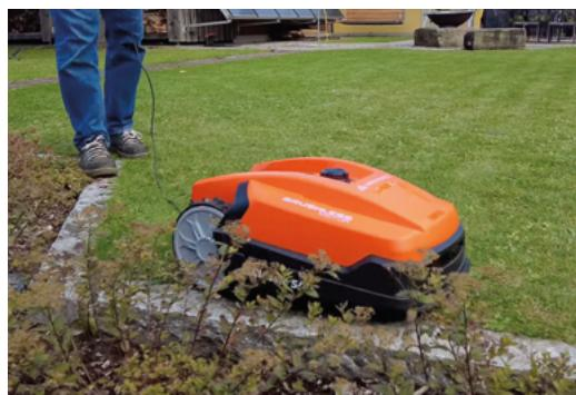
▲ By first driving the robot around the lawn perimeter, and obstacles such as trees, a GPS map is built up for automatic mowing
