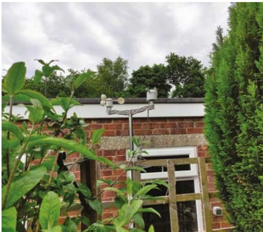
▲ Our weather station's cables go into the garage where a Weather HAT-equipped Raspberry Pi is located – an external weather-proof box would be better, however
