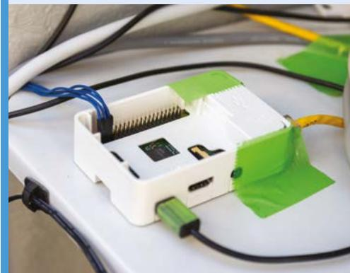
**02** A humidity monitor was set up for the telescope because the DAQ [data acquisition] system originally had no roof. A Raspberry Pi initiates the dome closure whenever humidity gets too high.
